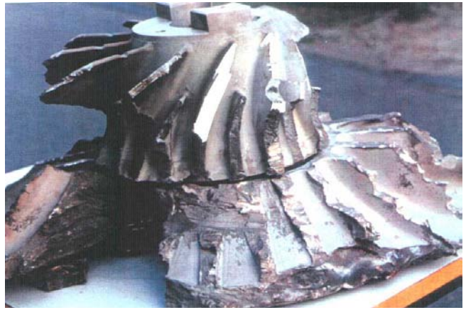
Fig. 99 Blower wheel of complete wrecked turbocharger (Author)
