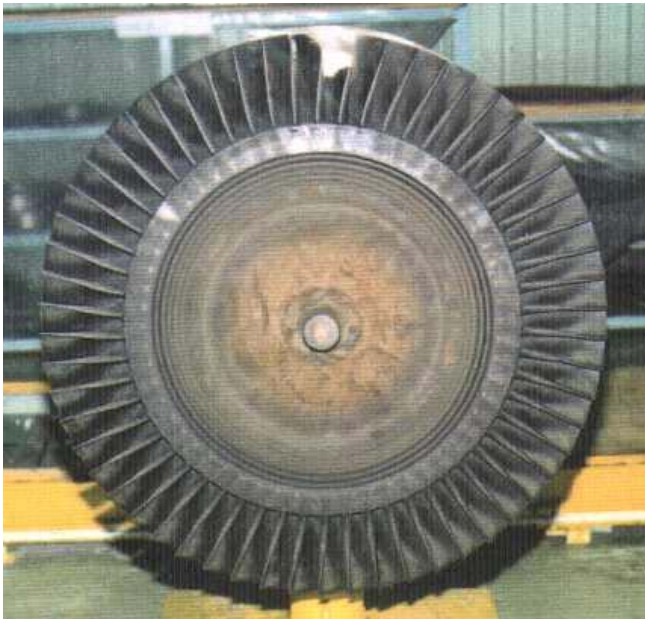
Fig. 98 Fatigue crack in turbine blade (Author)
