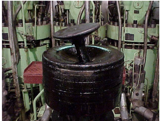
Fig. 116 Broken valve spindle forged through piston crown. (Author)
