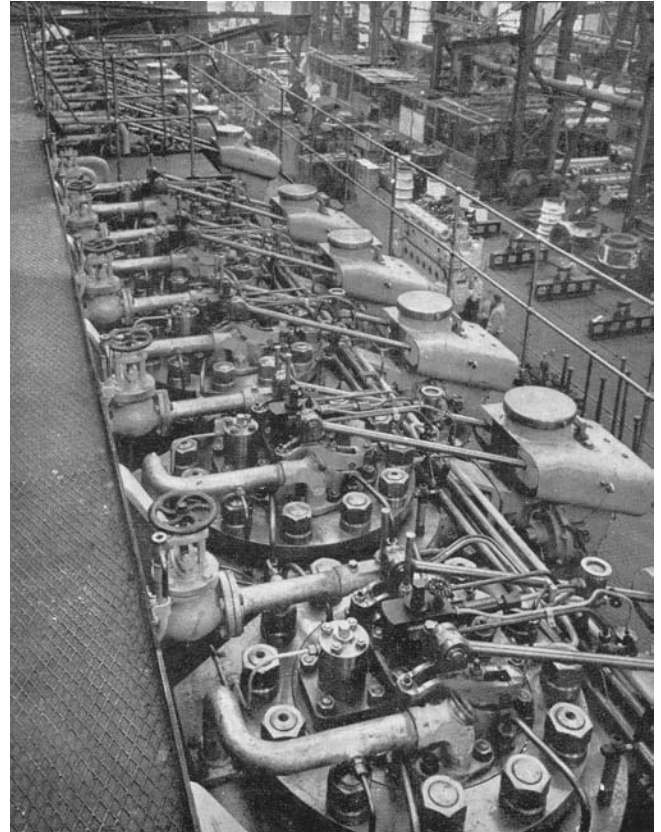
Fig. 9 KEBS68/125 engine top. Note the special exhaust valve gear. (MS [10])
