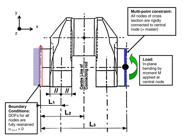
Figure 3.2 Boundary and load conditions for the pure bending load case.
