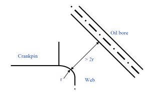
Figure 2.1. Oil bore proximity to fillet.
