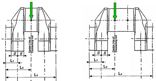
Figure 3.4 Load applications for in-line and V-type engines.
